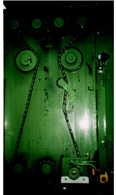
Tensioning of the chain drive system with SE-B 18 tensioner
