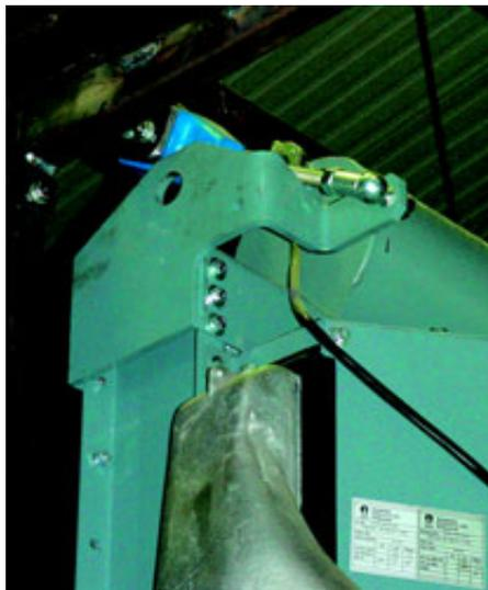
Fixation of water cooler with ST 38
