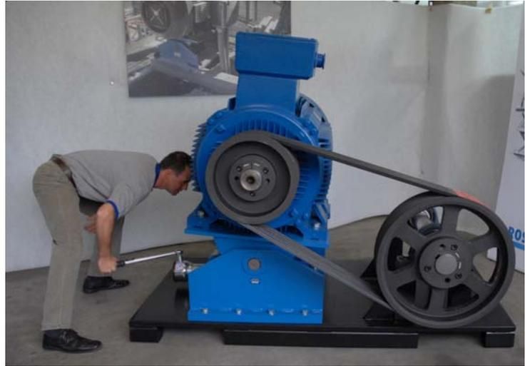
*Pretensioning of the 250 kW belt drive using a simple ratchet lever. The extremely light running bevel gear lifting spindle makes the easy handling of the ROSTA Type MB 100 motor drive possible without additional aids such as hydraulic cylinders, etc. The radial tensioning force required here for the six SPC drive-belts was 17,992 N!*
