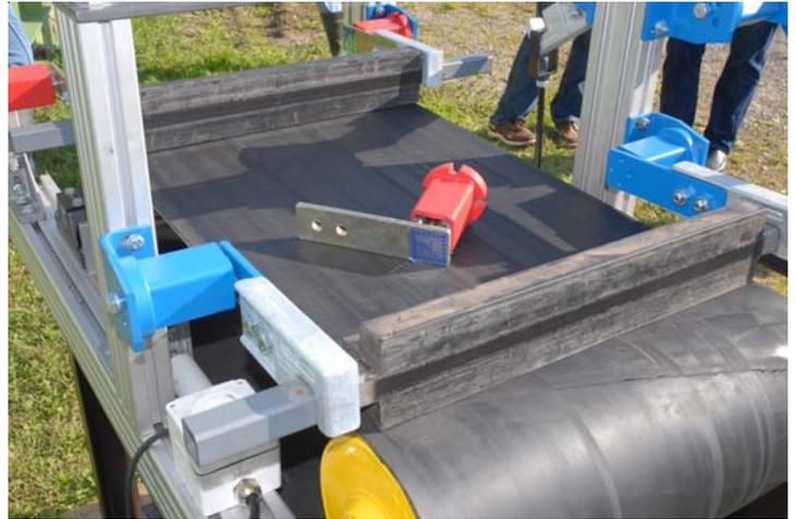
Suspension of crossover scrapers with ROSTA Type SE tensioning elements and, in comparison to the indefinable copy-tensioners that already "run-out" in practical trials after five minutes and no longer press the cleaning strips onto the belt.
