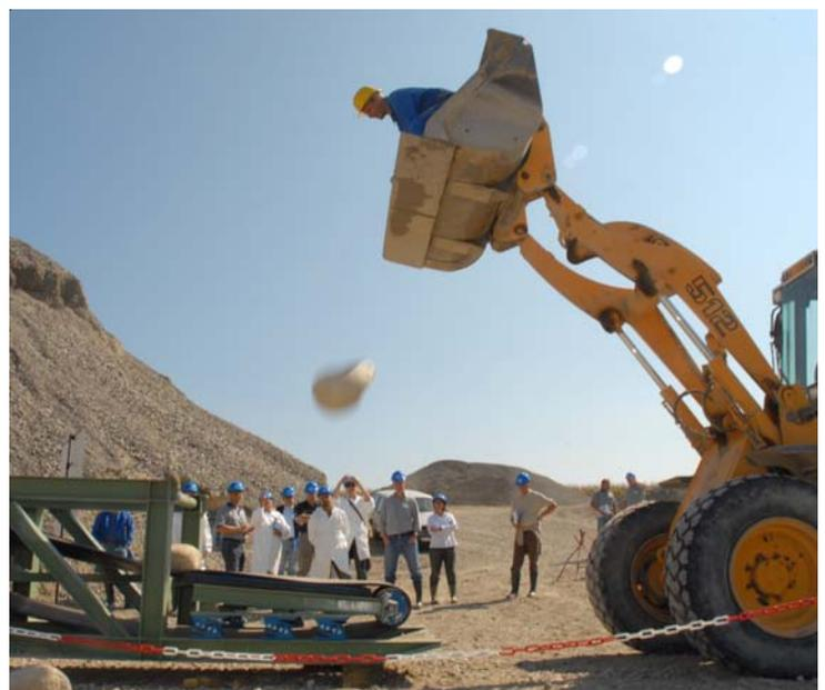
*Not all the sales technicians were convinced of the efficiency of the ROSTA Impact Table at the transfer stations. The sharp-edged 100 kg chunks falling from a height of 5 metres should prove the effectiveness of the ESL anti-vibration mountings. After thirty drops = not the slightest injury to the conveyor belt!*
