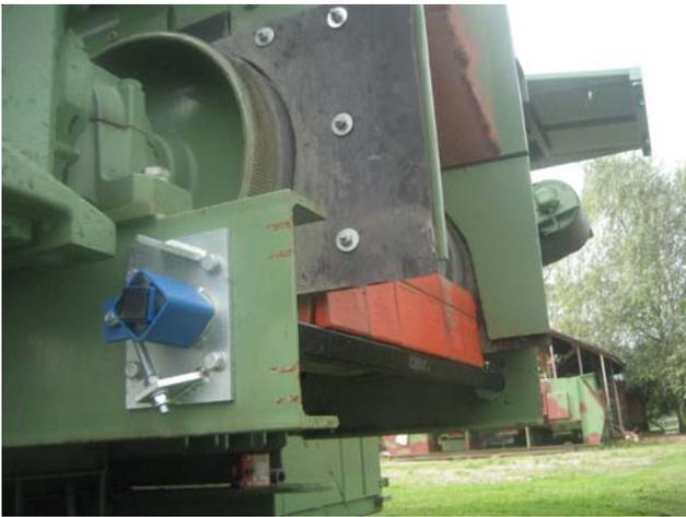
Demonstration of the new development of a self-adjusting ROSTA suspension system for the so-called drumhead scrapers. The Type DR 38 x 80 rubber suspension units that are fixed on both sides of the rubber belt frame can be synchronously pre-tensioned thanks to the tension scale and thereby provide an identical compression over the complete width of the belt.
