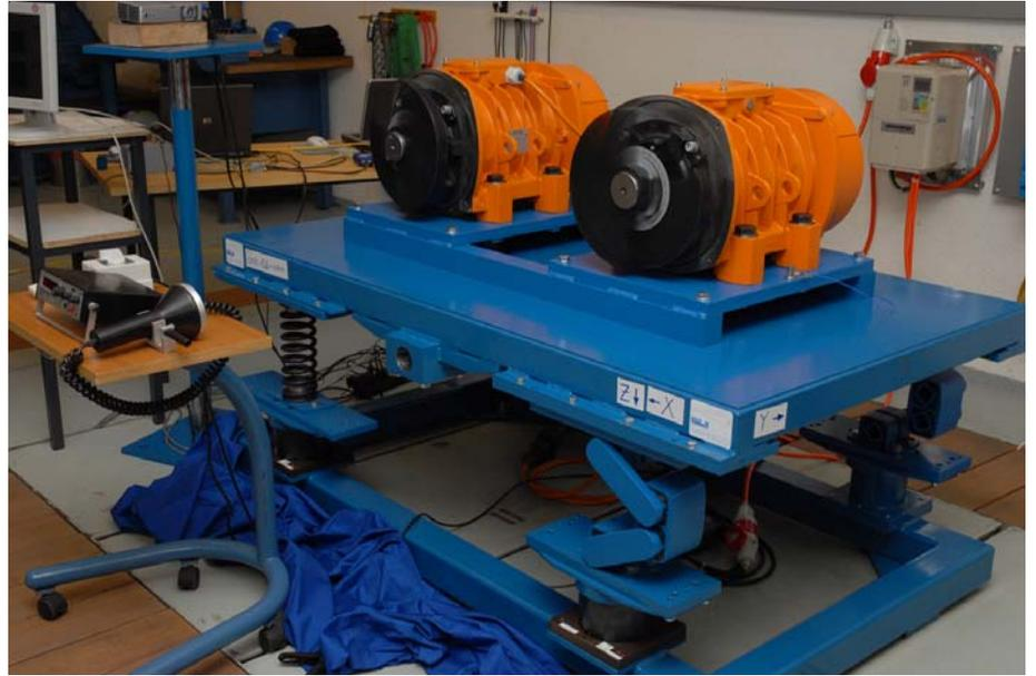
Even the measurement of the isolation efficiency was not forgotten! Do the ROSTA oscillating mountings really dissipate 98% of the vibrations? Yes, as much as 98.5% is “swallowed up” here by the ABs.
