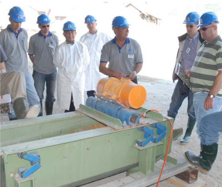
Do economic reasons suggest the use of the ROSTA pendulum mounts in linear screen drives with a single unbalanced motor? Yes, for small screening machines!
