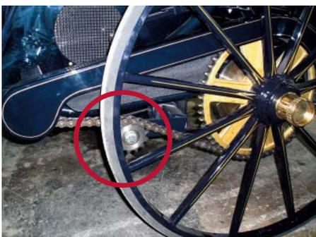
place by means of two 1" chains, which are tensioned using ROSTA SE 38 model tensioning elements. The chain wheels are mounted in a Z-arrangement, and a pretensioning angle of approx. 15° prevents any slapping of the loose side of the chain as well as compensating for the very high initial torque back lash when starting. Even after three years of driving, the drive and driven chain wheels (gear
