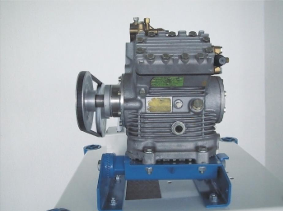
The motor base can be pre-tensioned up to a maximum angle of 30° using the two threaded shafts. The pre-tensioning of the torsion elements results in a very long compensation path for the take-up of the age elongation of the belt. In addition, the ROSTA rubber suspension elements also prevent the transmission of vibrations from the compressor to the vehicle chassis.
