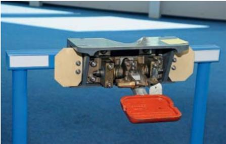
Almost all underground trains worldwide are equipped with elastic third-rail collectors to transfer power from laterally mounted tracks. The collectors themselves are mounted using ROSTA type DK 18 rubber suspension elements for elastic and vibration-free use. This application of the Blue Ones from ROSTA has proved itself since 1982.
