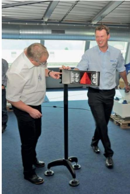
Using type DR 27 ROSTA elements, the elastically mounted and pivoting swivel taillights for lorry trailers reduce expensive rear light wear and tear when manoeuvring long lorry trailers. When the light beam deflects by 20°, an acoustic warning signal sounds in the driver's cab.
