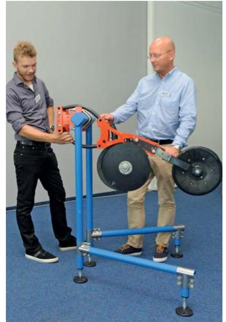
The planting of seeds using a multi-furrow seeding machine requires the immediate covering of the seeds so that a large portion of the seed does not become bird-feed. The rotary harrow with the furrow cover wheel has the necessary furrow cover pressure from a DR-27 spring parallelogram, which also compensates for uneven soil conditions (the two oscillating control arms, black).
