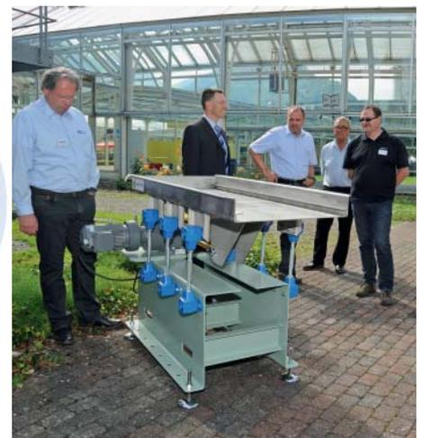
The conveyor trough with the revolutionary Shovel Drive (eccentric crank drive with three-times greater return speed) also demonstrated amazingly high conveying speeds even at low revolutions. These chutes can be designed to extend to a length of up to 40 meters.
