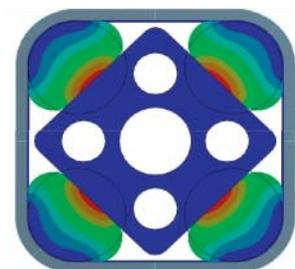
FEM-analysis of the ROSTA rubber suspension in idle mode
