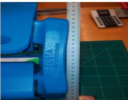
Test unit HS 50 after 10 times overload = slight deformation of the arms
