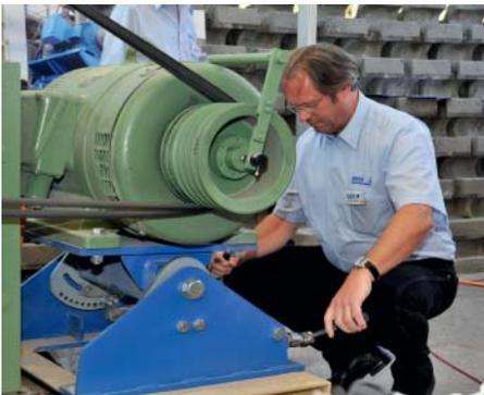
The "older and wiser heads" immediately understood the handling advantages of the new horizontal pre-tensioning device with trapezoidal screws on the MB 70
