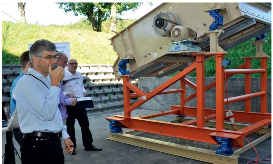
*Counter-mass frame (red) positioned on oscillating elements type AB-D 50*
