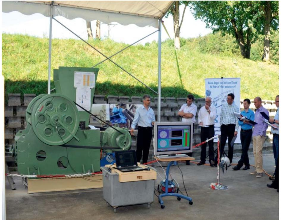
Drive motor for a jaw crusher, elastically positioned on a MB 70x550
