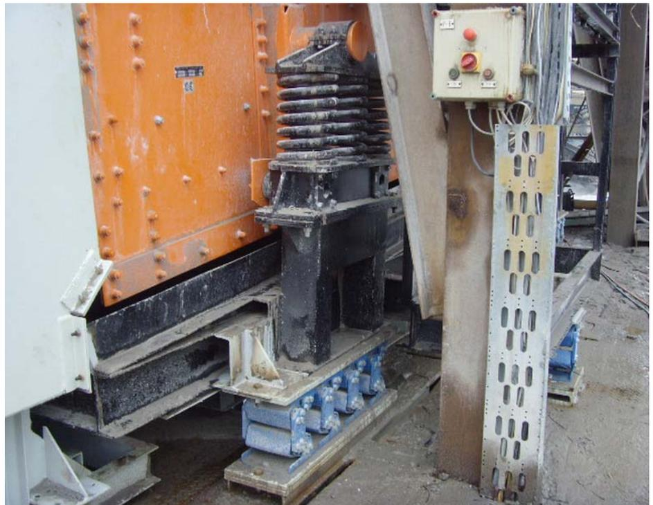
LZG screen with helical spring suspension, and the counterframe supported on 14 ROSTA Type AB-D 50-2 oscillating mountings
