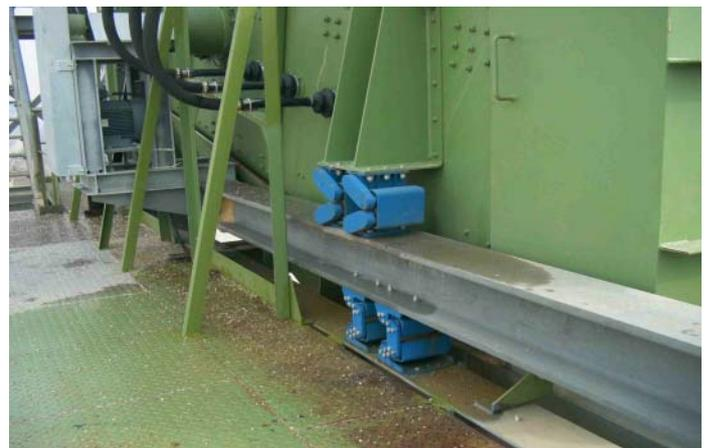
Cyros screen on a counterframe at a height of 30 m in the gravel works of Welbers GmbH, DE-Kevelaer
