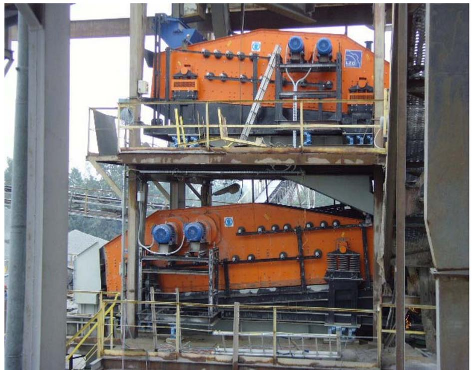
Two LZG linear vibratory screens on a counterframe with successive grain size selection (large grain outflow = upper screen; fine grain outflow = lower screen)
