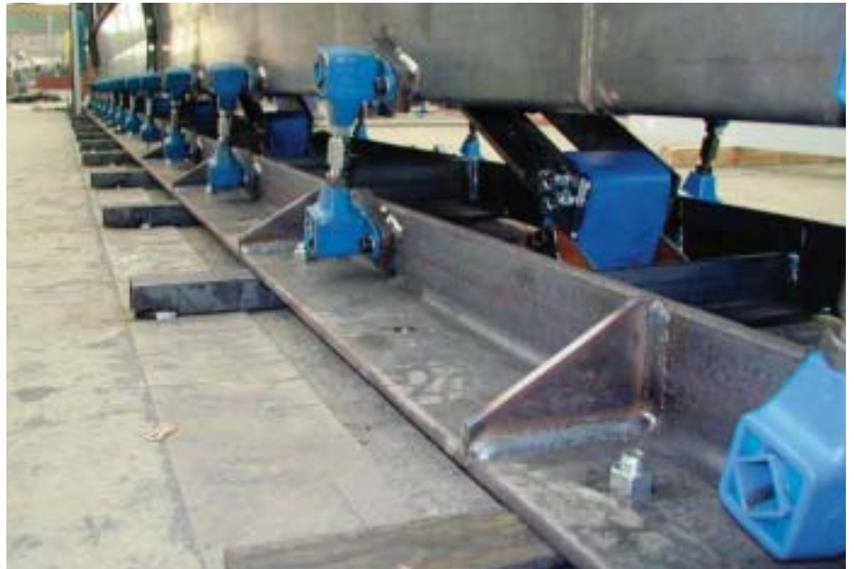
Single-mass resonance trough for castings with Type AU 45 oscillating mountings and DO-A spring accumulators
