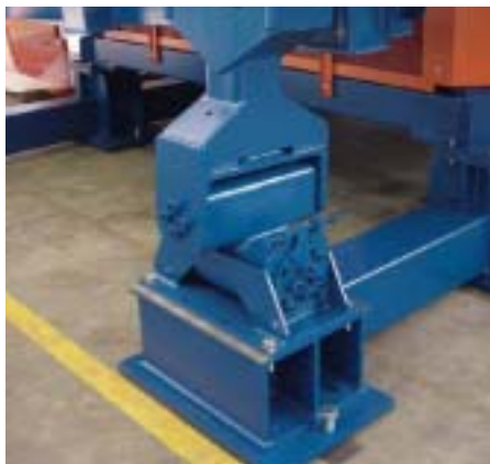
Gyrotory sifting machine suspension with universal joints, Type AK 100-4
