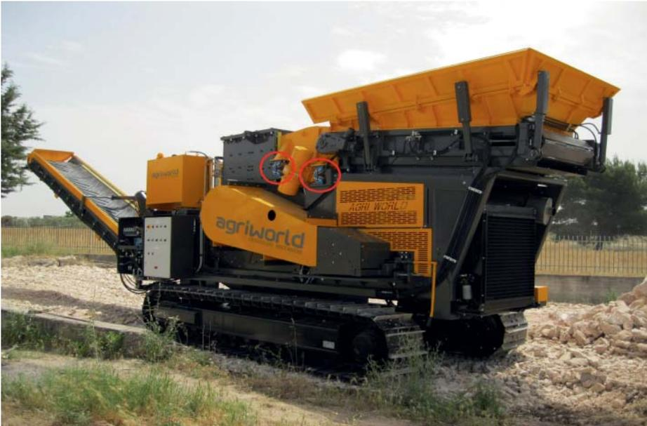
Mobile Crusher FM 9000.20, capacity 200 t/h
