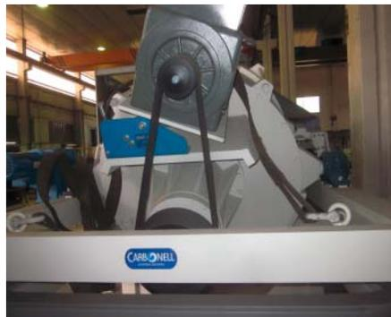
Drive motor for centrifuge installed on ROSTA Motorbase type MB 50x400
