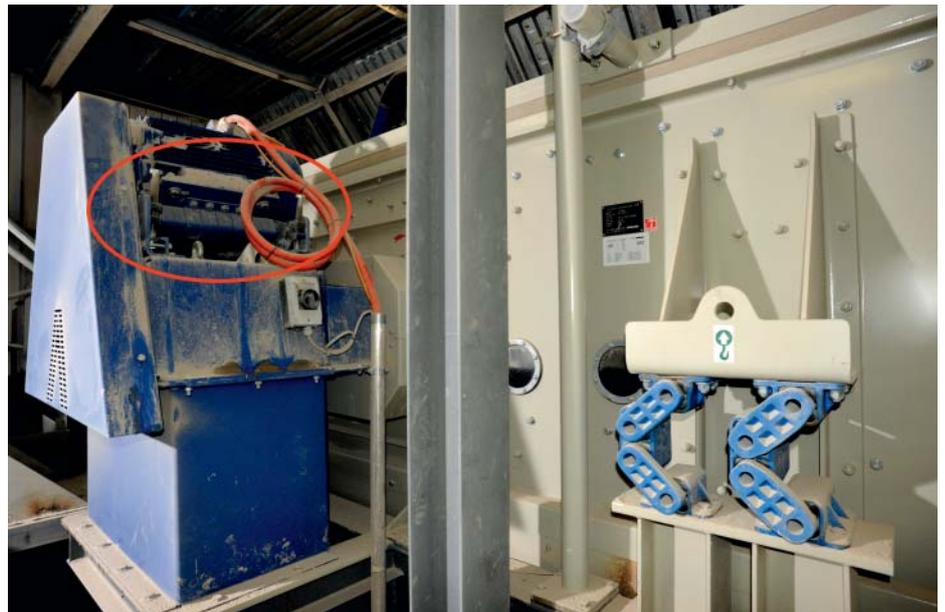
*Motor for belt transmission installed on ROSTA Motorbase type MB 50x270-2*
