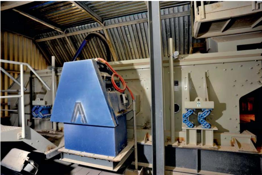
*Ammann elliptical motion screen mounted on AB-HD suspensions*
