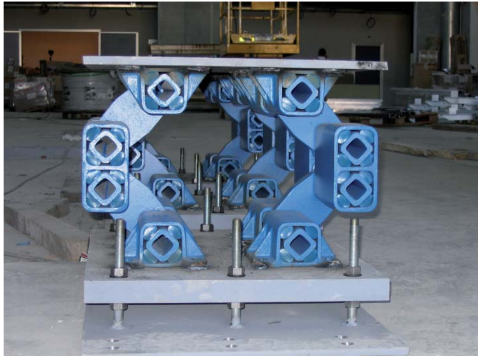
Nivelling „Sandwich-Plates“, each with 2 AB 50-2 TWIN supports
