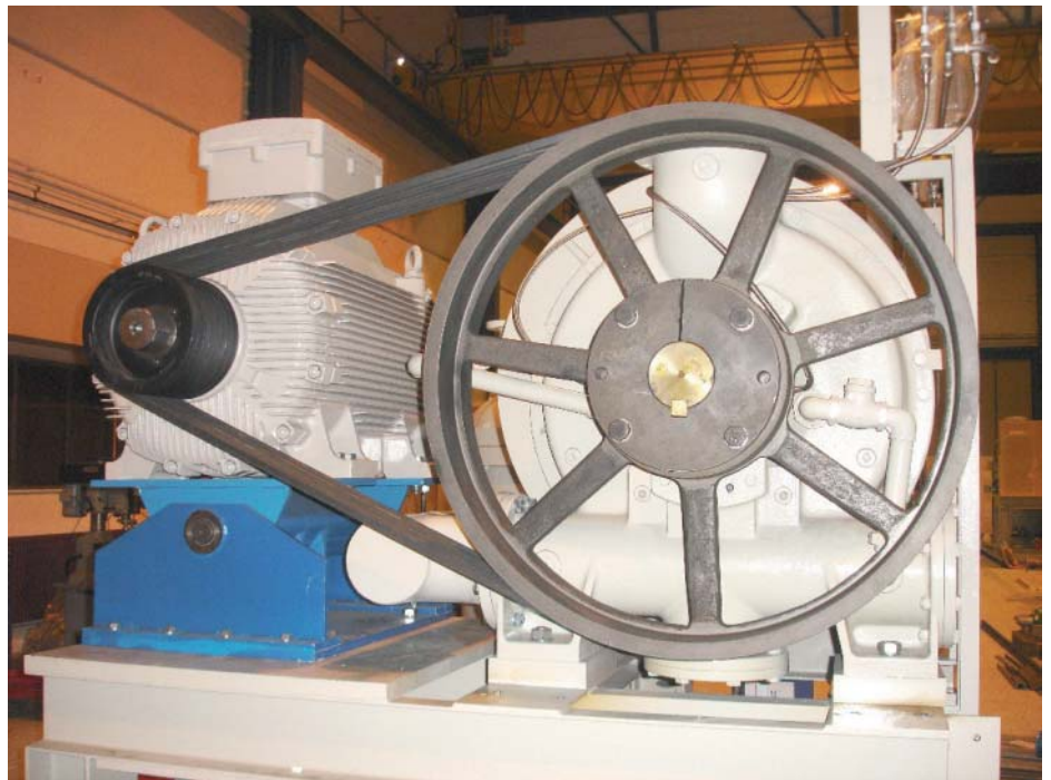
250 kW drive motor for the fluid ring pump on ROSTA Motorbase Type MB 100
