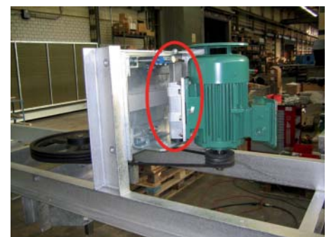
Belt drive for impeller ventilator mounted in vertical position on ROSTA Motorbase type MB 50 x 200
