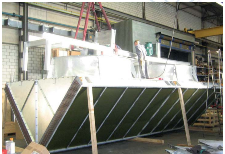
ECODYNE double block heat exchanger (V-shape) with two impeller ventilators for efficient air circulation
