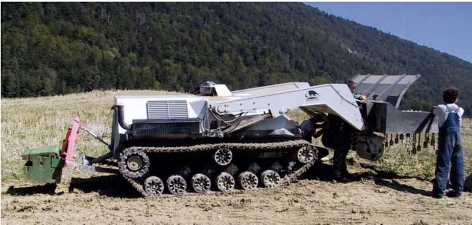
*Digger D-2 mine-clearing vehicle*
