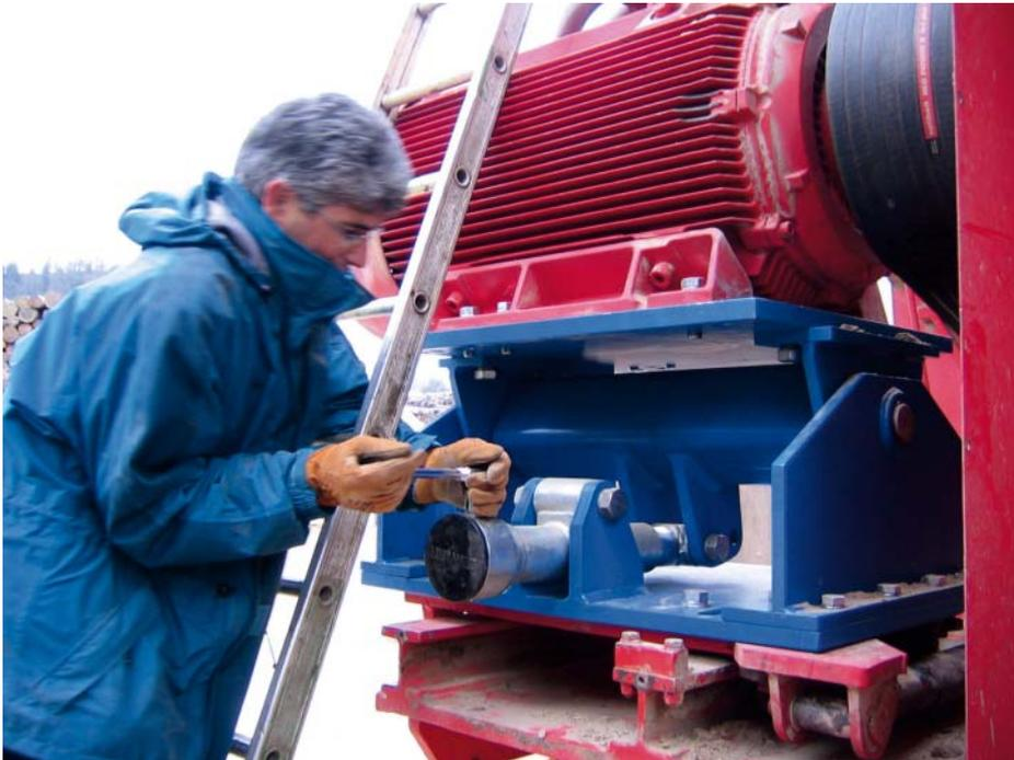
Tensioning the belt using a spindle gearbox
