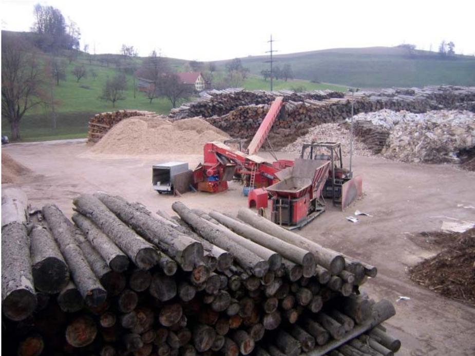
*Splintering chipper in the chipboard plant*
