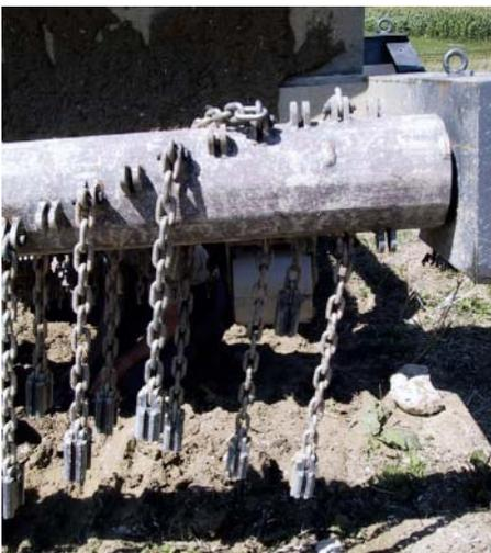
*Rotary chain-roller drum for triggering mines*
