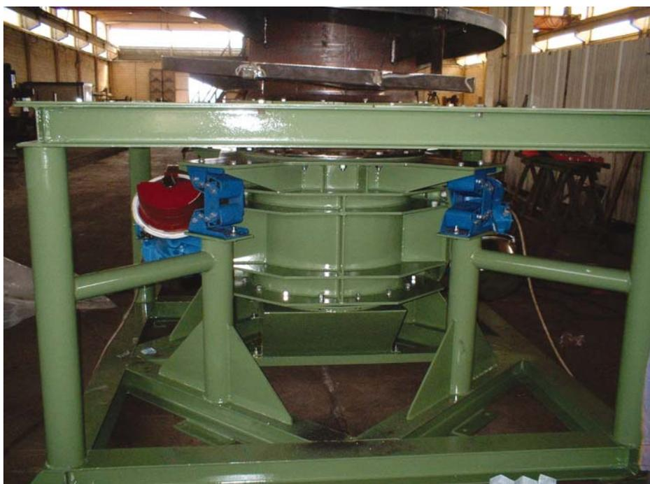
Drive using two 4 kW VENANZETTI vibration motors, 960 rpm. (Fig. 1)
