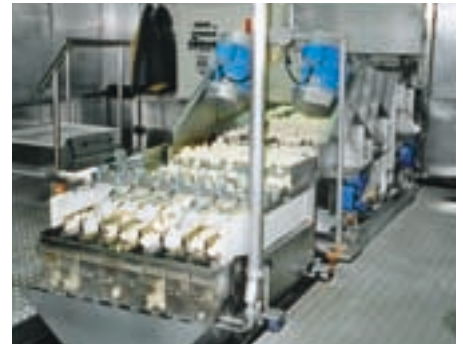
Lubbot-Wacker feeding and dewatering screen, originally equipped with coil spring mounts, retrofitted on ROSTA AB-45 oscillating mountings.
