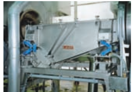
JÖST vegetable dewatering screen, originally coil spring suspension replaced by ROSTA AB-38 mounts
