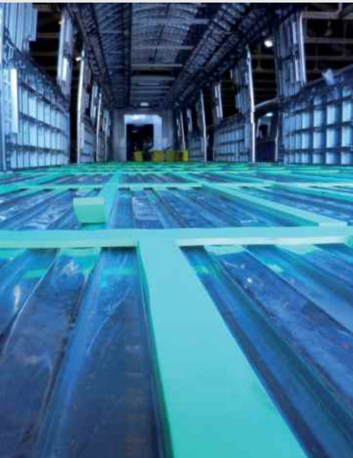
Floating floors for rolling stock
