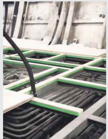
Decoupling of yacht flooring
